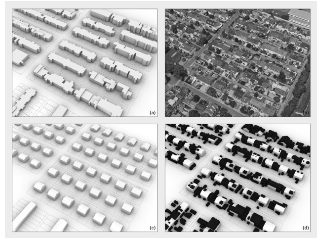
Figure 3. Four representations of the same part of Cité Ouvrière: (a) built volumes extruded according to the heights obtained by the photogrammetry, (b) Google 3D View, (c) built volumes of the area in 1897; and (d) final model integrating the original CO built volumes and their subsequent densifications.
